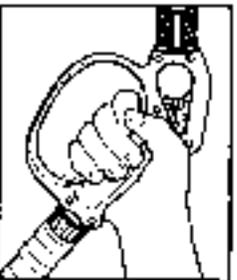
**Step 4** Trigger the gun to allow trapped air to wait for a steady flow of water to emerge from the spray nozzle.
